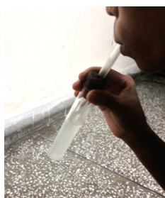
Fig. 6 : Lime Water Turning Milky
