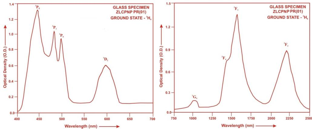
**Fig.2:** Absorption spectra of ZLCPNP (PR01) glass.
