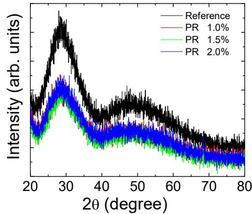
**Fig.1:** X-ray diffraction pattern of ZLCPNP (PR) glasses.
