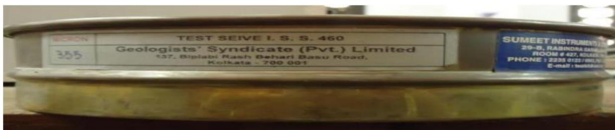
**Figure 1.1** 355  $\mu\text{m}$  sieve, used for sieving sample (powdered rice husk)
