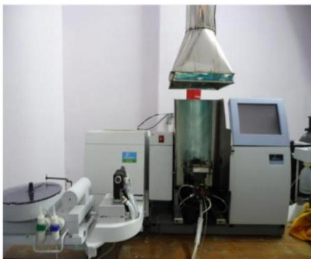
**Figure 1.4** Perkin-Elmer Model Analyst 200 atomic adsorption spectroscopy
