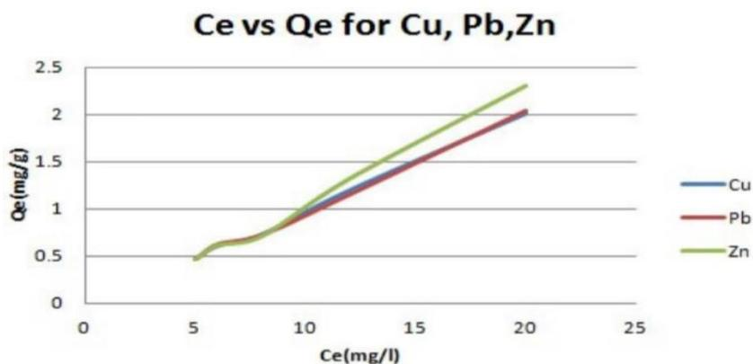
**Figure 1.7(a).** Effect of initial concentration of metals Zn, Cu, Pb on the adsorption capacity of carbonated rice husk (particle size < 355 micron)
