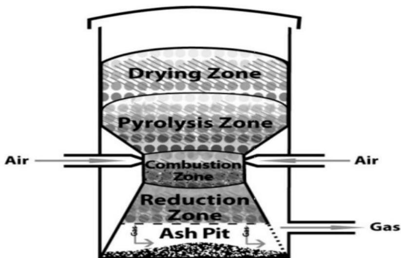
**Figure 1.9 Downdraft gasifier**
