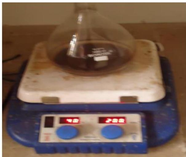
**Figure 1.5** Electromagnetic stirrer
