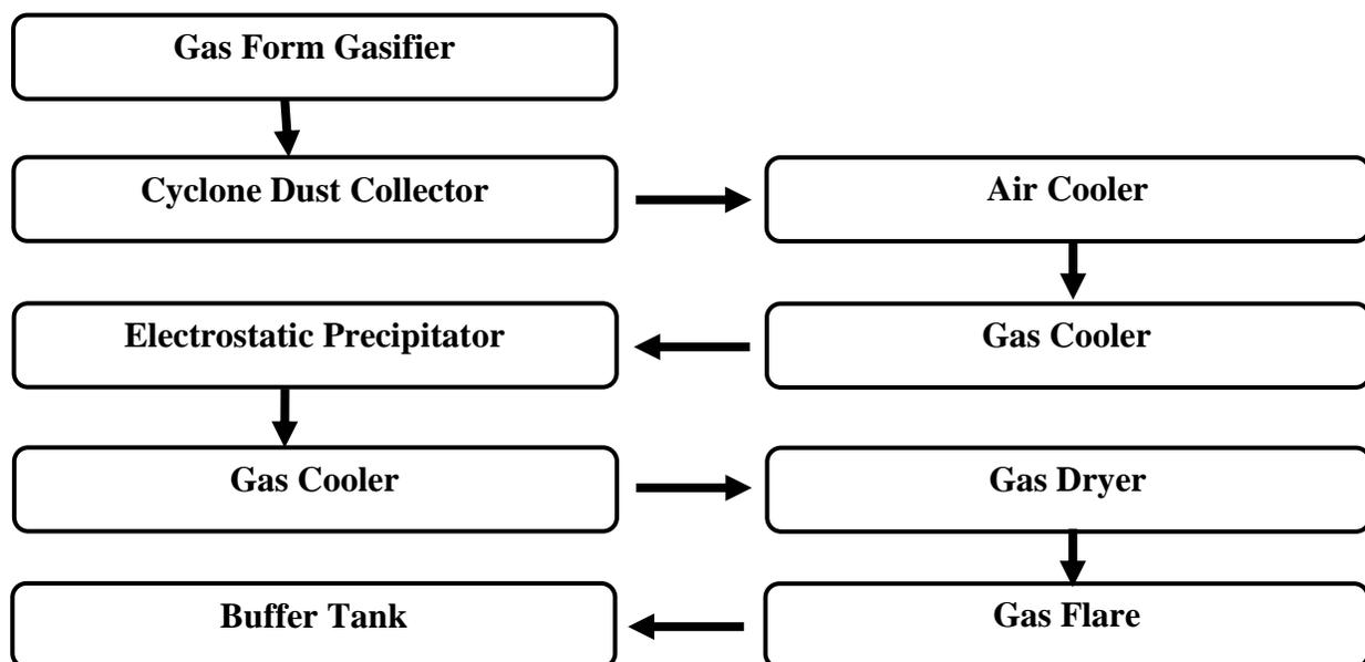
**Figure 1.10** Block diagram of purification unit
