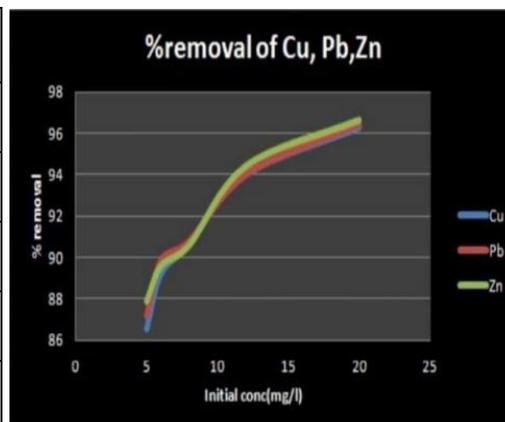
**Figure 1.7(b).** Graph between initial concentration of metals of the Zn, Cu, Pb and their respective % removal by carbonated rice husk.
