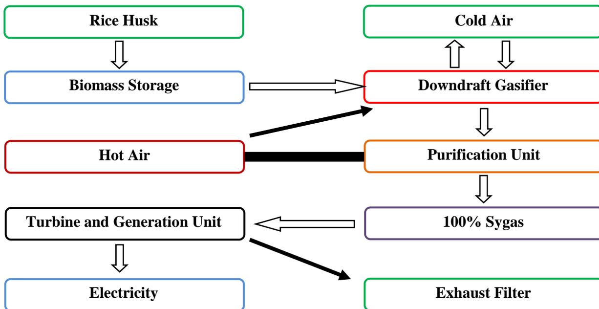
**Figure 1.8** Block diagram of rice husk electricity production unit
